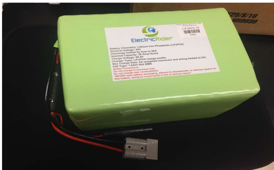
Figure 39. Custom LiFePO 4 Battery with BMS.
