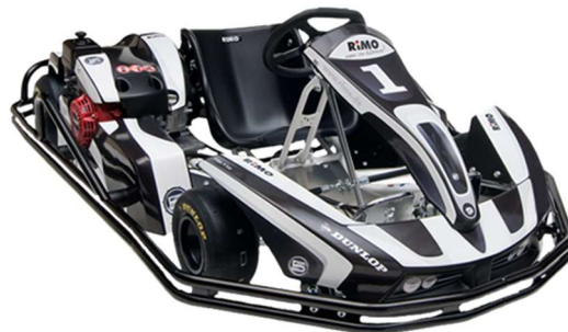
Figure 2. Go Kart with Chassis Designed to be Flexible.
